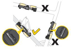
Make sure to install HybridRocket series pumps and CO<sub>2</sub> cartridges on Non-Drive side (left) downtube of bike only. The release arrow should be pointing towards the headtube.
